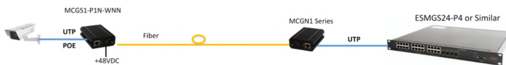
Typical Application -1: Point-to-Point Connection
