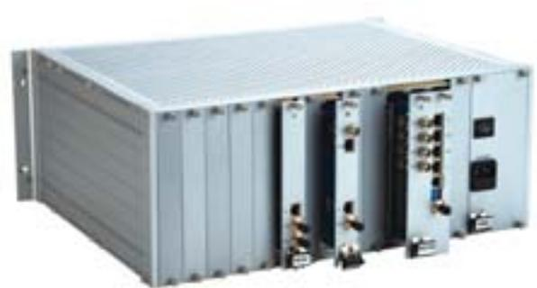
*Each ring uses two singlemode fibres, and at each node point, the ASFOM unit splits the signal electrically before transmitting through dual transmit and receive optics.*
