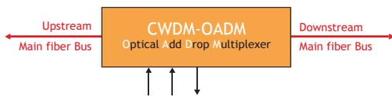
The remote end nodes on the bus system will have three optical connections - one each for the primary and secondary buses, and then a second or primary connection depending on the node's position in the bus. A CWDM device behind the single optical connections breaks the multiplexed link into the individual wavelengths used at that node.
