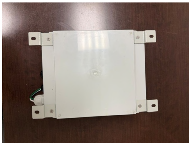
Figure 2 – Corner brackets fitted to the four corners of the back plate (rear view)
